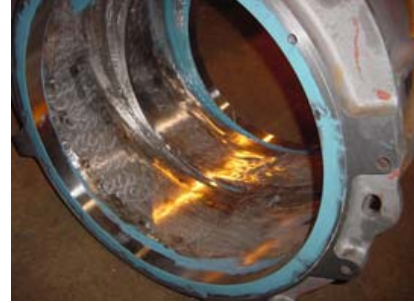
Inside of housing after cladding
