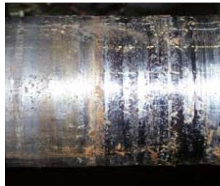
Shaft Needing Repair
