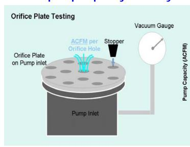
Vacuum Pump, Actual Cubic Feet / Minute, ACFM @ vacuum Measured by Orifice test method
