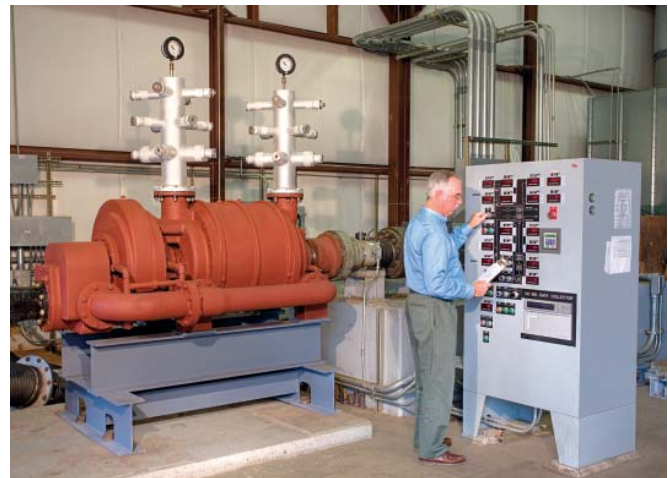
A Vooner FloGard high-vacuum two-stage pump being tested
